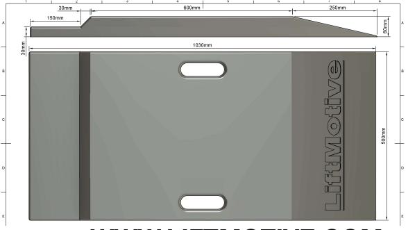
Dimensions: Lenght 1000mm, Width 500mm, Height 60mm Weight: 23,0 KG per Ramp
