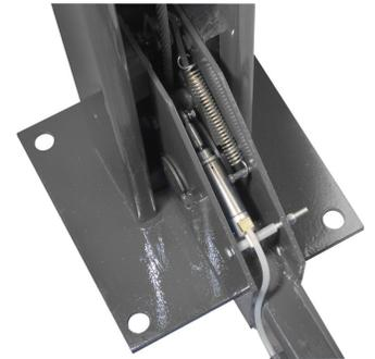
An air supply (minimum 30 psi / 3 CFM) is required for the safety-lock mechanisms to disengage. It is solely the responsibility of the end-user to provide, install and maintain the air supply.
